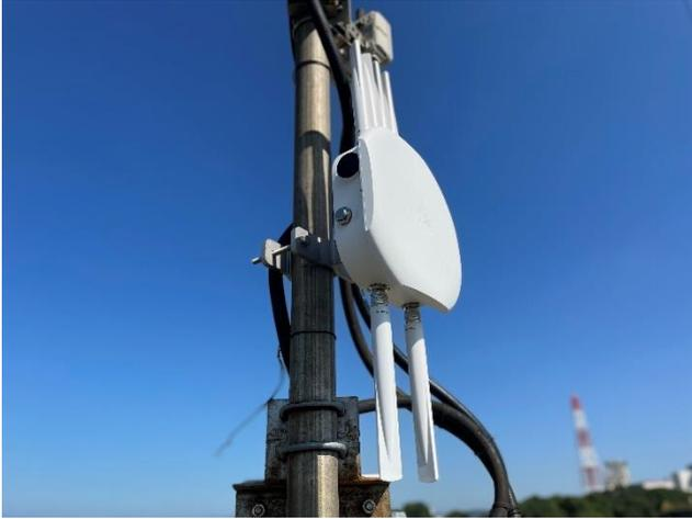
Prism MO10 Wi-Fi 6 AX6600 Tri-Radio Outdoor Mesh Router is housed in a rugged IP68 aluminum enclosure. The casing provides the waterproof, dustproof, wind load and salt spray protection against the extreme environment conditions in the air.
